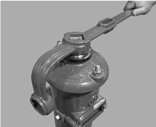
13. Use the operating wrench to check for proper operation of the indicator. Verify that the "OPEN" target plate is completely visible in the window when the valve is in the fully open position. Verify that the "CLOSED" target plate is completely visible in the window when the valve is in the fully closed position.
