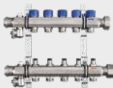
Manifold - Equipped with air bleeder Model 2878.914, purge valve Model 2878.915, supply shutoff balancing valve Model 2878.924 - Stainless steel - SVC, union connection, female pipe thread - Preassembled Model 2879
