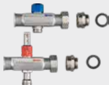
Manifold expansion set - For stainless steel manifold shutoff / balancing / flow meter - Suitable for manifold Model 2804, manifold ball valve set Model 2877.2 - Stainless steel - Union connection, female pipe thread Components (2) 1 1/4" MPT x 1" MPT adapter, (2) gaskets, (2) expansion nipples Model 2877.5
