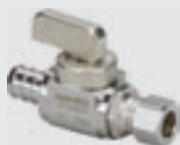
Viega PEX Crimp Stop valve Straight Zero Lead - Equipped with ferrule Model V5085, Viega PEXC rimp ring Model V5019.9 - Chrome-plated brass - Crimp connection - 1/4 turn Model V5026ZL
