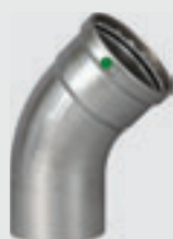
Viega ProPress Elbow 45° XL, street Smart Connect feature, Zero Lead - Stainless steel 316 - Press connection, male copper tube size Components EPDM sealing element Model 4026.1XL
