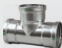
Viega ProPress Tee XL Smart Connect feature, Zero Lead - Stainless steel 316 - Press connection Components EPDM sealing elements Model 4018XL
