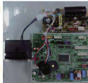
Connection of terminal block and Main PBA
