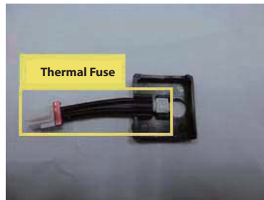
Terminal Block Internals
