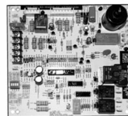
INTEGRATED FURNACE CONTROL
