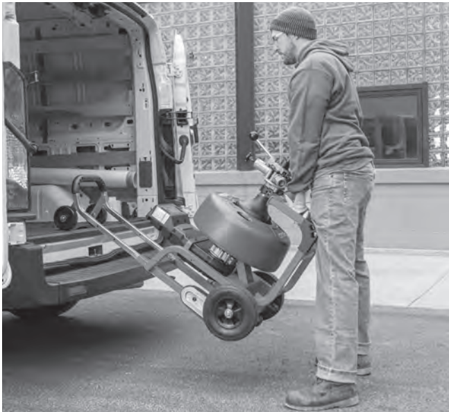
Figure 26 – Loading on a Vehicle
