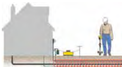
Direct connect to utility lines.
