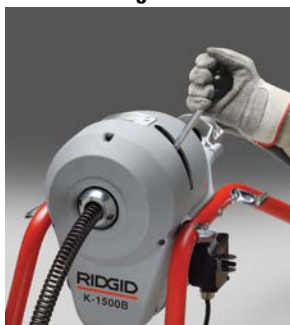
Engage clutch, cable spins.
