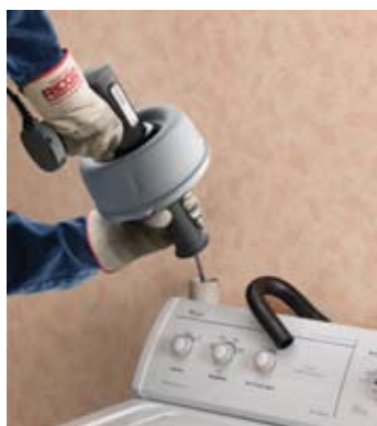
The 3/8" cable in the K-39AF-5 and K-39AF-7 extends machine's capacity to 2 1/2" drain lines.
