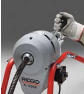
Engage clutch, cable spins.
