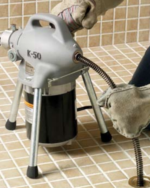
K-50 – The Professional's choice since 1957 because of its power and versatility. Use 5/8" cables for 1-1/4" to 4" lines. Add the A-17 adapter for 3/4" to 2" sink lines.
