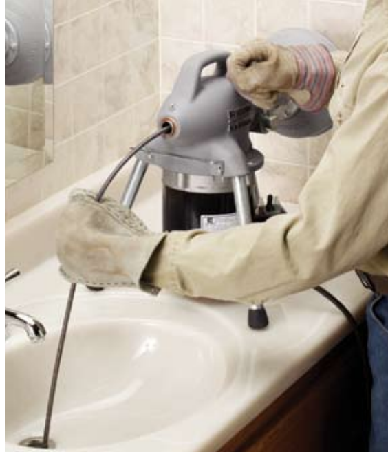
K-50 – The Professional's choice since 1957 because of its power and versatility. Use 5/8" cables for 1-1/4" to 4" lines. Add the A-17 adapter for 3/4" to 2" sink lines.
