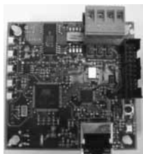
BACnet® COMMUNICATION CARD RXRX-AY01
