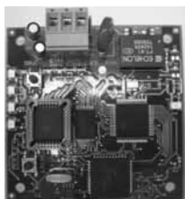
LonWorks® COMMUNICATION CARD RXRX-AY02
