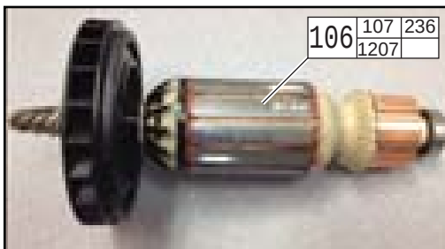
#106, No. 16-10-0137 Armature Assembly (Armature, fan and rear ball bearing) with Crank Assembly #236
