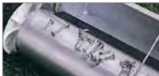
Quick Release rotates housing toward hopper.
