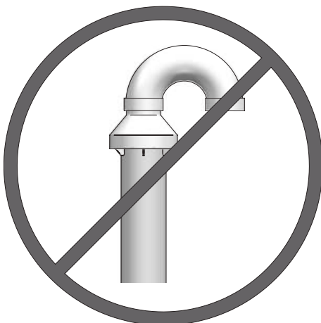
Figure 4-5 Do Not Install U-Bent to Rain Cap
