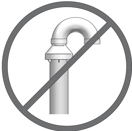
Figure 5-5 Do Not Install U-Bend to Rain Cap
