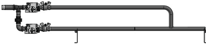
Figure 8-5 _Gas Train 500,000 Btu/hr Model
