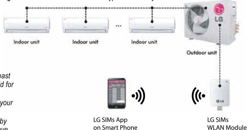
Figure 78: SIMs WLAN Module to a Typical Multi F System
