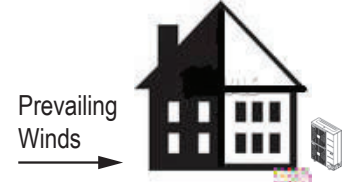
Figure 28: Leeward Side of the Building.
