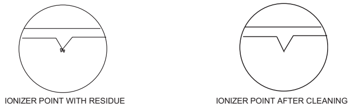
Fig. 19. Removal of deposits from ionization points.
