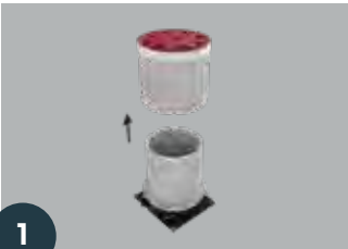
1 Cut inner and outer sleeve if desired height is under 8"
