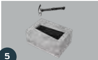
Remove styrofoam & "knock out plug"
