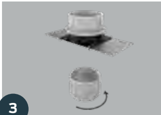
3 Install inverted outer sleeve to bottom of base
