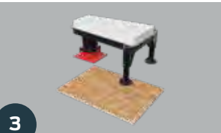
Nail tub box to form deck
