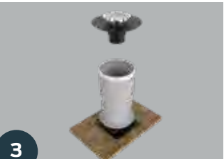
3 Set drain on top of sleeve
