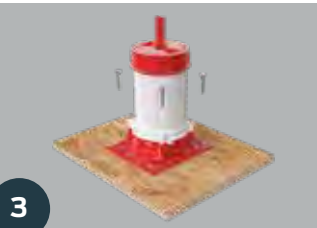
3 Nail to form deck
