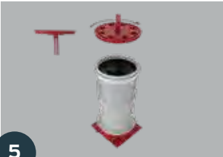
5 Re-install cap & insert whiskers
