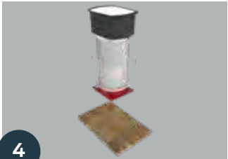
4 Nail to form deck
