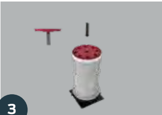
3 Re-install cap & insert whiskers
