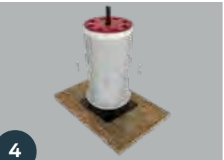
4 Nail to form deck
