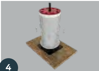
4 Nail to form deck
