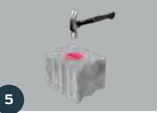
5 Knock out safety cap with hammer or screwdriver
