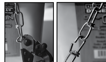
Cut with Duro Dyne Cable Cutter
