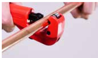
1. Cut the tube to length
