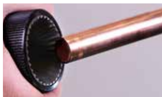
2. Deburr and remove all external sharp edges
