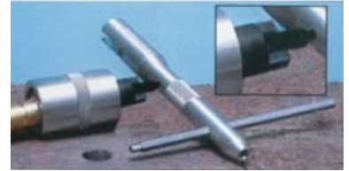
Step 6: Place square tip of stud into tool to remove old anchor from extractor.
