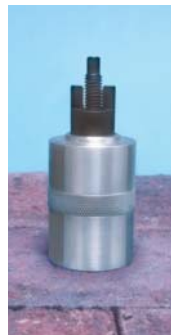
Step 4: Thread castle nut onto extractor.
