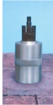
Step 4: Thread castle nut onto extractor.
