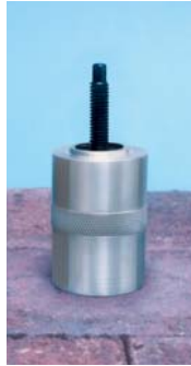
Step 3: Place extractor over stud.
