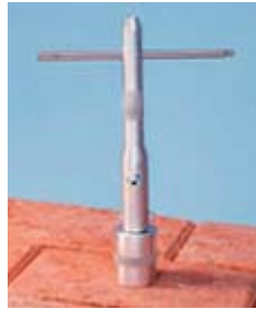
Step 5: Place tool on castle nut and turn clockwise to remove anchor.
