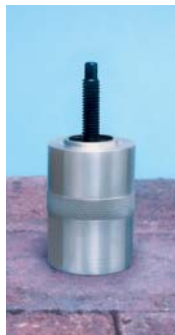
Step 3: Place extractor over stud.
