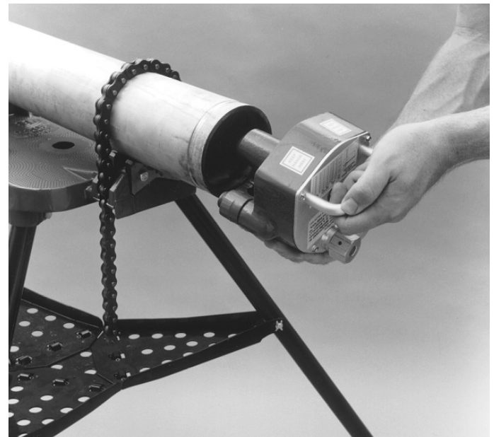
Fig. 6. Dismounting the tool.
